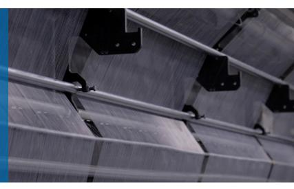
The reinforcement scrim layer serves as a main source of membrane strength in our reinforced material. Knitted in-house, Plastatech's anti-wicking polyester weft-insertion scrim has either an 18 by 14 or 18 by 9 threads per inch density. This enhanced thread density and high tensile strength provided by the polyester yarn offers superior puncture resistance, while the weft-inserted tie yarn prevents tears from spreading.
